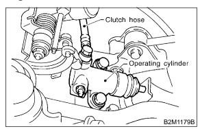
3) Remove operating cylinder from transmission.
