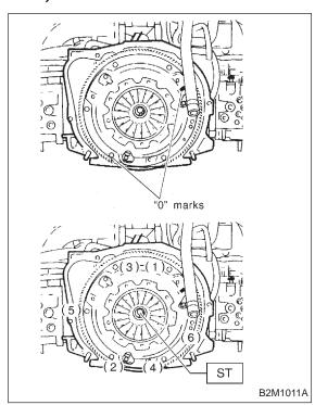
5) Remove ST. ST 499747100 CLUTCH DISC GUIDE
