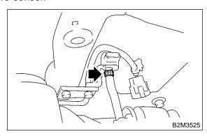
7) Remove fuel tank pressure sensor.
