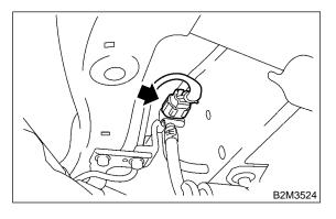
6) Disconnect pressure hose from fuel tank pressure sensor.
