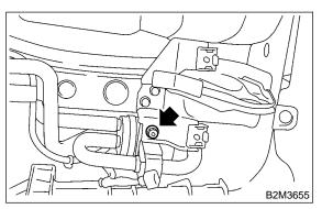
7) Disconnect evaporation hoses, and remove drain filter.
