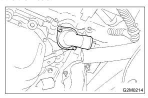
6) Install the thermostat in the water pump, and install the thermostat cover together with a gasket.
