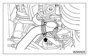
5) Remove thermostat cover and gasket, and pull out the thermostat.
