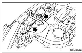
7) Install air intake duct.
