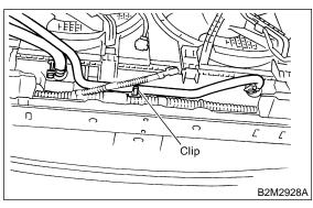
10) Connect connectors to radiator main fan motor and sub fan motor.
