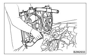
3) Install radiator brackets and tighten bolts.
