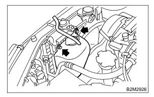
12) Disconnect radiator inlet hose from engine.
