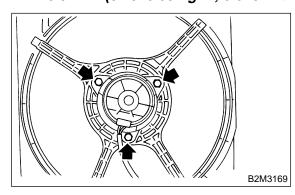
Tightening torque: 3.4±0.5 N⋅m (0.35±0.05 kg-m, 2.5±0.4 ft-lb)
