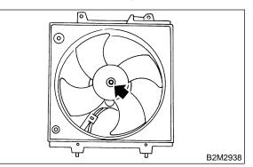
3) Remove bolts which install fan motor onto shroud.
