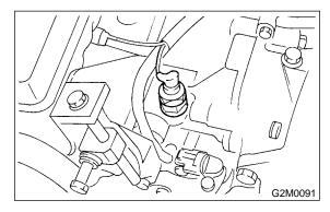
3) Remove oil pressure switch.
