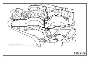
7) Connect connector and terminal to generator.
