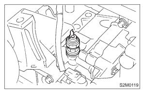
3) Connect terminal of oil pressure switch.
