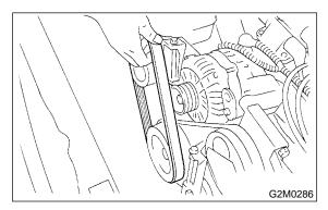
(4) Remove bolts which install generator on bracket.
