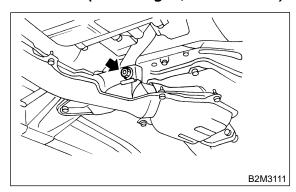
8) Connect rear oxygen sensor connector.
