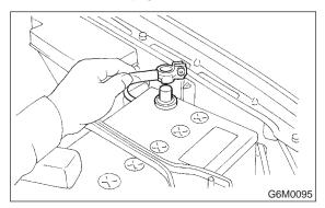
2) Disconnect front oxygen (A/F) sensor connector.
