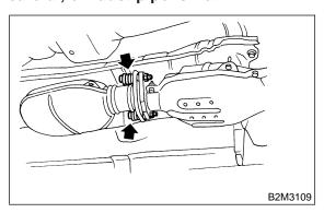
2) Separate rear exhaust pipe from muffler.
