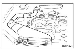
5) Disconnect connector from intake air temperature sensor. (MT vehicles)
