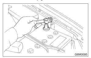
2) Remove bolts which install air intake duct on the front side of body.
