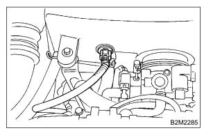
6) Loosen clamp which connects air cleaner case to throttle body.
