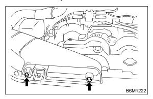
3) Remove bolt which installs air intake duct on body.
