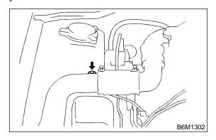
4) Remove air intake ducts as a unit.
