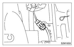
4) Remove knock sensor from cylinder block.
