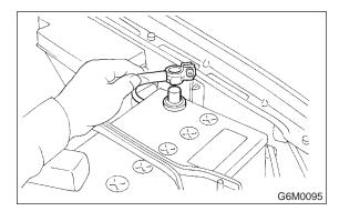
2) Disconnect connector from front oxygen (A/F) sensor.
