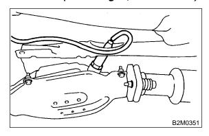
3) Connect connector to rear oxygen sensor.
