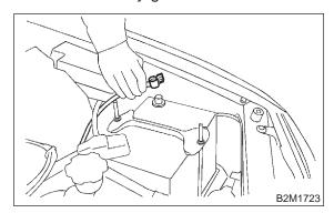
2) Disconnect connector from rear oxygen sensor.
