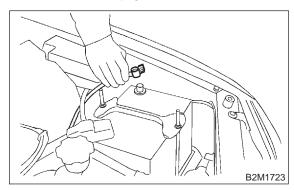
2) Remove idle air control solenoid valve. <Ref. to 2-7 [W15A1].>
