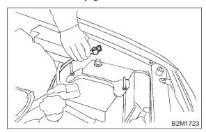
2) Disconnect connector from intake air temperature sensor.
