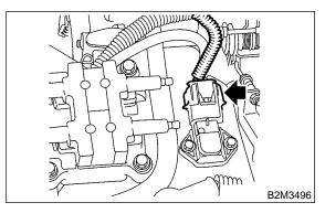
4) Remove intake air temperature and pressure sensor.
