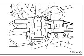
3) Disconnect connector from intake air temperature and pressure sensor.
