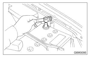
2) Disconnect connector from atmospheric pressure sensor.
