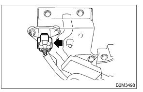
3) Remove atmospheric pressure sensor from bracket.
