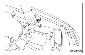
2) Disconnect connector from idle air control solenoid valve.
