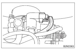
3) Disconnect air by-pass hose from idle air control solenoid valve.
