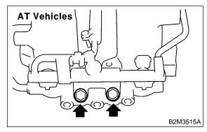
Tightening torque: T1: 18.6±1.5 N⋅m (1.9±0.15 kg-m, 13.7±1.1 ft-lb)
