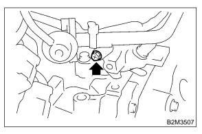
11) Remove fuel injector from intake manifold.(1) Remove fuel injector securing clip. (AT vehicle)
