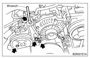
(5) Disconnect connector from power steering pump switch.
