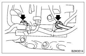
13) Remove bolt which holds injector pipe to intake manifold. (AT vehicles)
