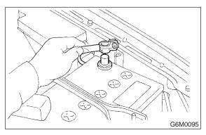
4) Remove two bolts which install washer tank on body.
