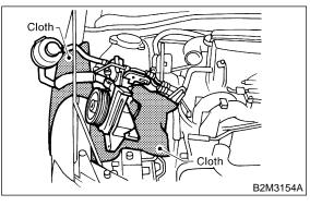
8) Remove intake manifold protector RH.
