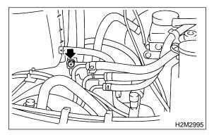
16) Remove fuel injector from intake manifold.(1) Remove fuel injector securing clip. (AT vehicles)
