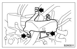
11) Remove intake manifold protector LH.
