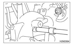
15) Remove bolt which holds fuel pipe on the left side intake manifold.
