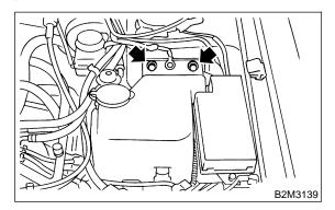
5) Disconnect connector from front window washer motor.
