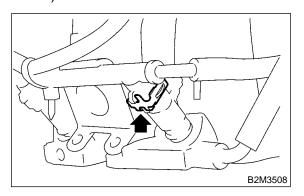
(2) Remove fuel injector while lifting up fuel injector pipe.
