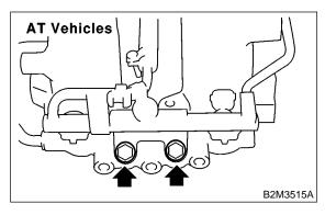
14) Remove bolt which installs injector pipe to intake manifold.
