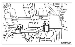
(4) Remove bolts which install power steering pump to bracket.
