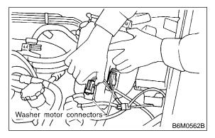
7) Disconnect rear window glass washer hose from washer motor, then plug connection with a suitable cap.
