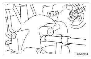
Tightening torque: 4.9±0.5 N⋅m (0.5±0.05 kg-m, 3.6±0.4 ft-lb)
