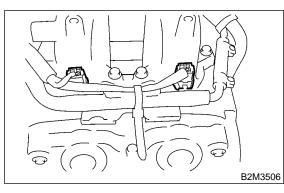
10) Remove bolt which install injector pipe to intake manifold.
