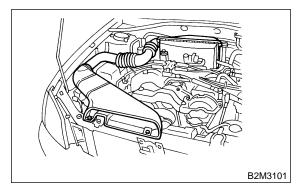
5) Remove resonator chamber.
