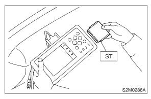
4) Connect Subaru Select Monitor to data link connector.
