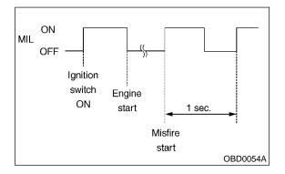
4) When ignition switch is turned to ON (engine off) or to "START" with the test mode connector connected, the MIL blinks at a cycle of 3 Hz.
