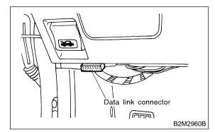
3) Using the OBD-II general scan tool, call up diagnostic trouble code(s) and freeze frame data. OBD-II general scan tool functions consist of:
