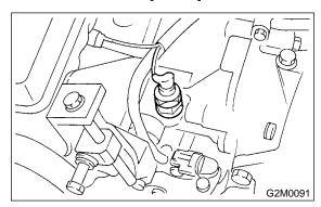
5) Connect oil pressure gauge hose to cylinder block.
