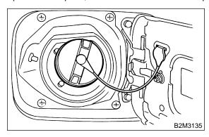
3) Disconnect fuel delivery hoses from fuel filter, and connect fuel pressure gauge.
