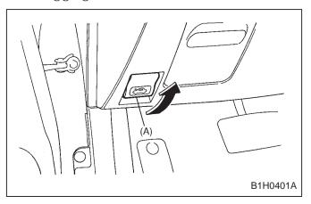
2) Release the lock by pushing the lock lever (A) while pushing the hood down with slight pressure.
