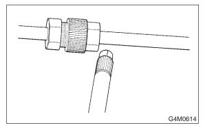
3) Check the area of the pressure switch (dual switch), and also check the seams of the receiver drier.
