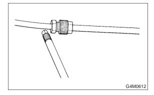
• Check the area where the two parts of the fitting join each other.
