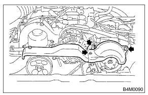
3) Check that clearance between drive plate and pulley over the entire perimeter is within specifications.
