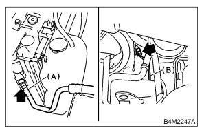
5) Remove the radiator bracket (A).
