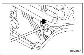
7) The condenser should be installed in the reverse order in which it was removed. When installing the condenser, pay attention to the following:
