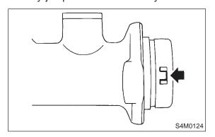
4) Extract primary piston assembly and secondary piston assembly.
