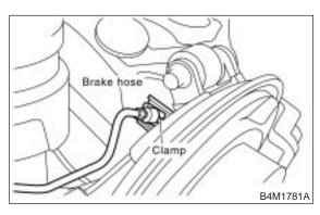
2) Pull out clamp to remove brake hose.
