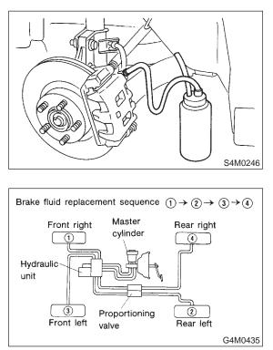
3) Slowly depress the brake pedal and keep it depressed. Then, open the air bleeder to discharge air together with the fluid.
