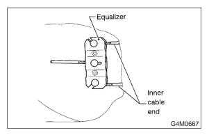
11) Pull out parking brake cable from rear brake. <Ref. to 4-4 [W3A0].> or <Ref. to 4-4 [W4A0].> 12) Pull out clamp from rear brake.
