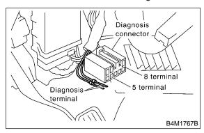
2) Repeat 3 times within approx. 12 seconds; connecting and disconnecting terminal 8 and diagnosis terminal for at least 0.2 seconds each time.
