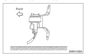
CHECK : Is the voltage between 3.7 and 4.1 V when G sensor is inclined forwards to 90°?
