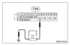
(CHECK): Is the resistance less than 0.5  $\Omega$ ?
