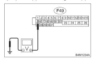
(CHECK): Is the voltage between 10 and 17 V?
