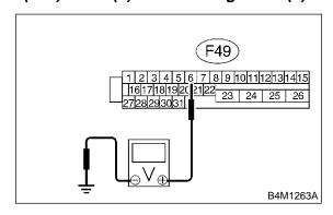
: Is the voltage less than 1 V? CHECK
