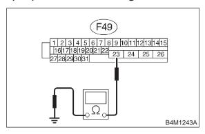
(CHECK): Is the resistance less than 0.5  $\Omega$ ?
