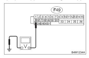
CHECK): Is the voltage between 10 and 15 V?
