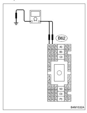
CHECK : Is the resistance less than 0.5  $\Omega$ ?
