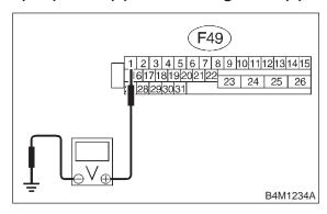
CHECK): Is the voltage between 10 and 15 V?
