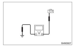
(CHECK): Is the voltage less than 1 V?
