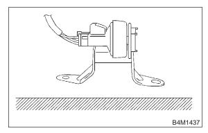
CHECK : Is the voltage between 2.1 and 2.4 V when G sensor is horizontal?
