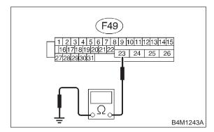
(CHECK): Is the resistance less than 0.5  $\Omega$ ?
