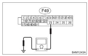
: Is the resistance less than 0.5  $\Omega$ ? CHECK)
