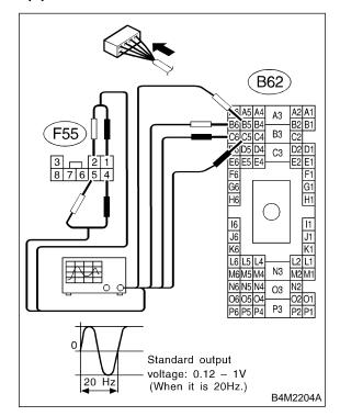
CHECK : Is oscilloscope pattern smooth, as shown in figure?
