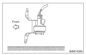
CHECK : Is the voltage between 0.5 and 0.9 V when G sensor is inclined backwards to 90°?
