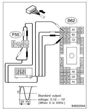
CHECK : Is oscilloscope pattern smooth, as shown in figure?
