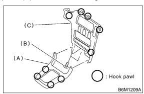
6) Remove fitting screws, and slightly pull radio bracket out from center console while disconnecting connector.
