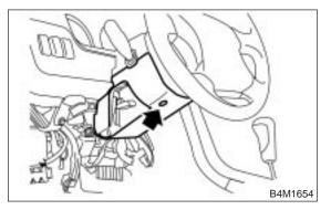
8) Remove all connectors from steering column.9) Remove the two bolts under instrument panel securing steering column.
