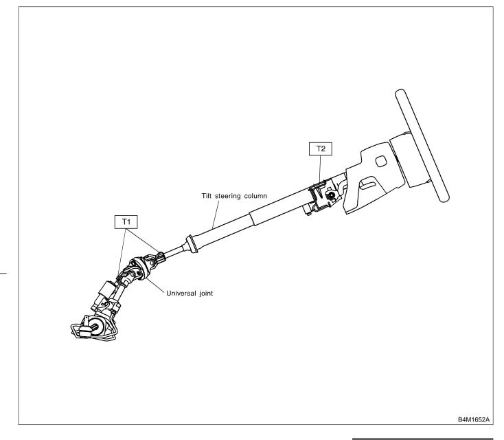
Tightening torque: N·m (kg-m, ft-lb) T1: 24±3 (2.4±0.3, 17.4±2.2) T2: 25±5 (2.5±0.5, 18.1±3.6)
