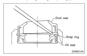
3) Pry off oil seal using screwdriver.
