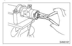
8) Fit mounting rubber onto rack housing.
