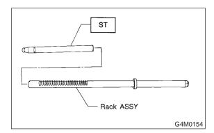
3) Apply genuine grease to teeth of thoroughly washed rack assembly, and fit ST over the toothed portion.
