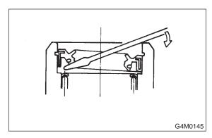
4) Press-fit oil seal into valve housing using ST and press.
