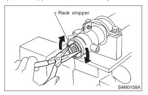
2) Pull rack assembly from cylinder side, and draw out rack bushing and rack stopper together with rack assembly.
