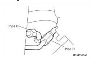
6) Remove bolt A. Disconnect pipe C from oil pump. Disconnect pipe D from return hose.
