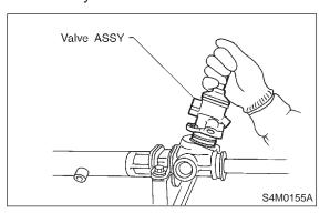
3) Tighten bolts alternately to secure valve assembly.
