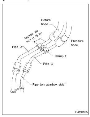
6) Temporarily install clamp E on pipes C and D.
