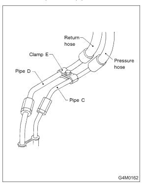
5) Disconnect pipe C·D from pipe (on the gearbox side).
