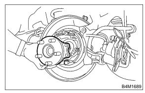
If it is hard to remove, use STs. ST1 926470000 AXLE SHAFT PULLER ST2 927140000 PLATE
