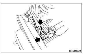
7) Remove brake caliper from back plate and suspend it from stabilizer using a piece of wire.
