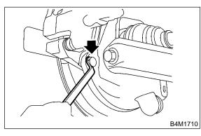
8) Install rear ABS sensor and brake cable bracket.
