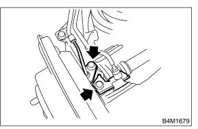
9) Adjust parking brake lever stroke by turning adjuster. <Ref. to 4-4 [W9B0].>
