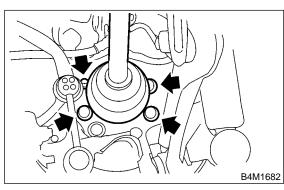
10) Remove hub unit bearing.
