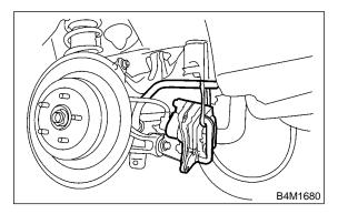
8) Remove disc rotor from hub.
