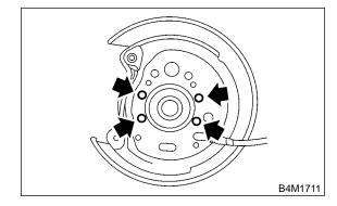
2) Tighten four bolts to back plate.
