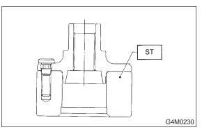
2) Using ST1, ST2 and ST3, press hub unit bearing into hub.
