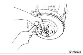
12) Install wheel and tighten wheel nuts to specified torque.
