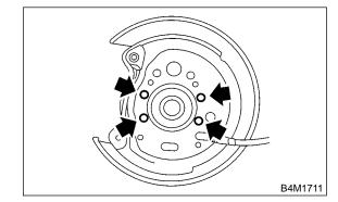
2) Tighten four bolts to back plate.
