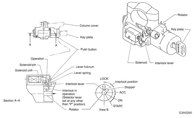
• When the selector lever is moved to "P", P position switch in the selector lever assembly turned ON, and the solenoid pin moves to the release position so that the lever spring disengages the interlock lever from the rotator's stopper. As a result, the key plate can be rotated to the "LOCK" position. The key plate can be inserted into or removed from the "LOCK" position only.
