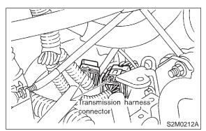
3) Check each sensor, solenoid and ground system for short circuits.
