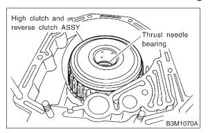
14) Take out the high clutch hub and the thrust bearing.
