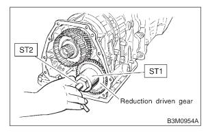
(3) Using the ST, extract the reduction drive gear.
