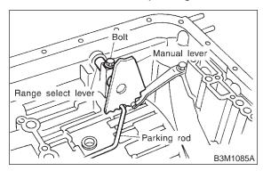
7) Insert spring pin to manual lever.
