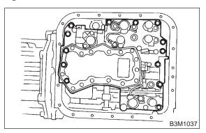
9) Remove vehicle speed sensor 2 (front) and torque converter turbine speed sensor.
