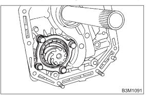
(3) Install the oil pump housing assembly to the torque converter clutch case, and secure evenly by tightening four bolts.
