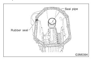
2) Install the torque converter clutch case assembly to the transmission case assembly, and secure with six bolts and four nuts.
