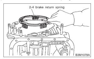
22) Take out 2-4 brake piston and piston retainer.
