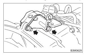
9) Tighten the drain plugs.
