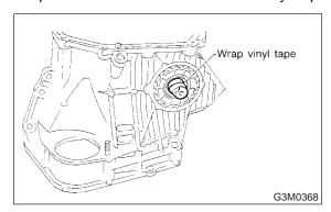
2) Remove the differential side retainer with ST.
