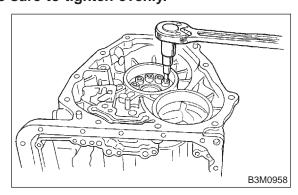
(4) Install thrust needle bearing.
