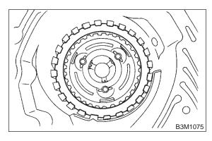
19) Take out the thrust needle bearing, planetary gear assembly and the low clutch assembly.
