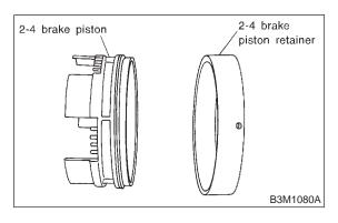
16) Install 2-4 brake piston and retainer to transmission case.
