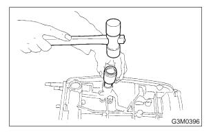
2) Install parking support to transmission case.
