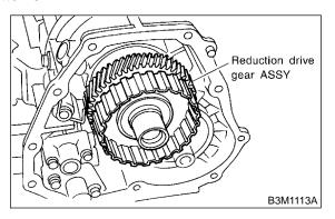
6) Using a plastic hammer, install reduction driven gear assembly, and tighten drive pinion lock nut.
