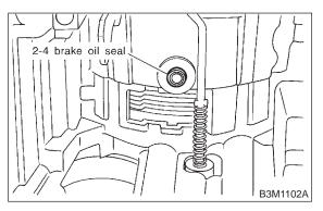
(3) After all 2-4 brake component parts have been installed, blow in air intermittently and confirm the operation of the brake.
