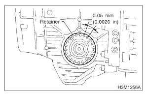
(7) Turn the drive pinion several rotations with ST1 and check to see if the backlash is within the standard value with ST2, ST3, ST4 and ST5.
