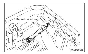
5) Insert range select lever, and tighten bolt.
