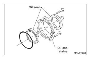
11) Attach the O-ring to the oil seal retainer with vaseline. Install the seal to the oil pump housing bore.
