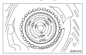
23) Install front sun gear and thrust needle bearing.
