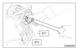
4) Remove the differential case assembly.
