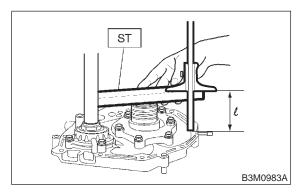
(3) Calculation of total end play Select suitable bearing race from among those listed in this table so that clearance C is in the 0.25 — 0.55 mm (0.0098 — 0.0217 in) range. C = (L + G)  $-\ell$
