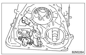
4) Connect connector to duty solenoid C (transfer).
