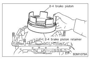
23) Separate 2-4 brake piston and piston retainer.
