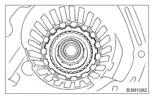
27) Turning the case upside down, take out the one-way clutch inner race, retainer and wave spring.
