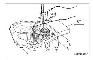
(2) Measure the distance " $\ell$ " from the transmission case mating surface to the reduction drive gear end surface with ST1 and ST2.
