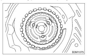
(2) Install 2-4 brake oil seal to transmission case.
