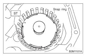
19) Install planetary gear and low clutch assembly to transmission case.
