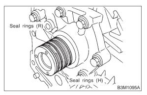
14) Install the rubber seal to the torque converter clutch case.
