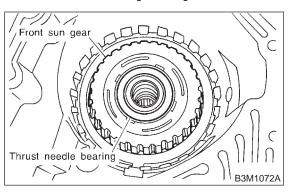
24) Install the high clutch hub and thrust needle bearing.
