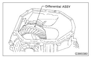
4) Install the circlip to the axle shaft, insert the shaft into the differential assembly, and tap it into position with a plastic hammer.
