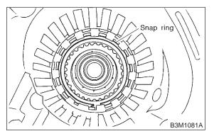
26) Take out retaining plate, drive plate, driven plate and dish plate.
