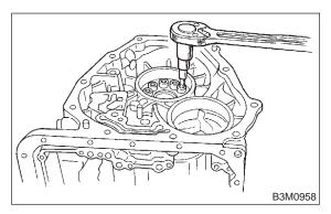
28) Take out the low & reverse piston by applying compressed air.
