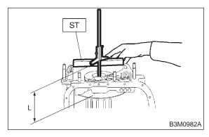
(2) Using ST, measure the distance from the oil pump housing mating surface to the top surface of the oil pump cover with thrust needle bearing. ST 398643600 GAUGE
