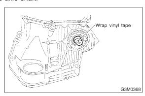
6) Install the oil seal and outer race (taper roller bearing) to the differential side retainer. Then screw in the retainer and the O-ring after coating the threads with oil.
