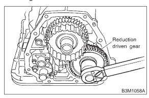
(2) Using the ST1 and ST2, extract the reduction driven gear.
