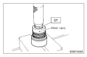
(2) Install two seal rings to one-way clutch inner race.
