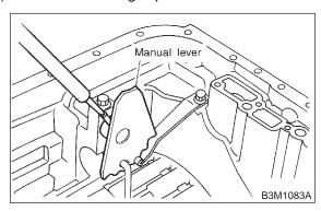
31) Remove bolts securing select lever, then remove select lever, manual lever and parking rod.
