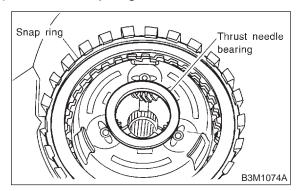
18) Take out retaining plate, drive plate and driven plate of 2-4 brake.
