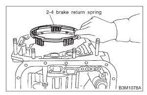
18) Position snap ring in transmission. Using ST, press the snap ring into place.
