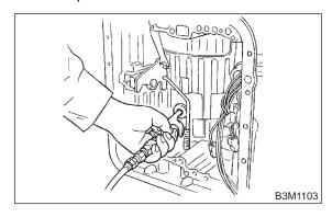
(4) Measure the clearance between the retaining plate and the snap ring.
