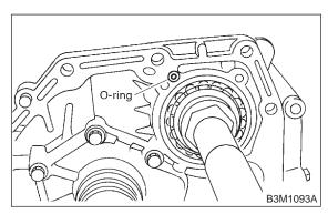
12) Install the oil seal retainer taking care not to damage the oil seal lips. Then secure with three bolts.
