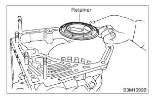
11) Install the one-way clutch inner race.
