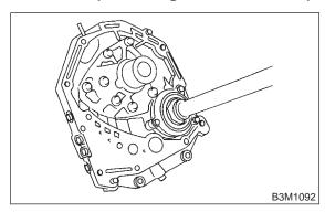
(4) Rotate the drive pinion several times with ST1 and ST2.
