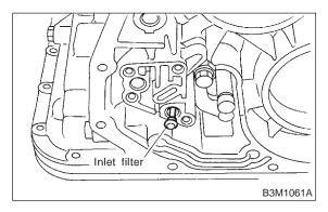
3) Install transfer valve plate, valve body and duty solenoid C (transfer) to transmission case.
