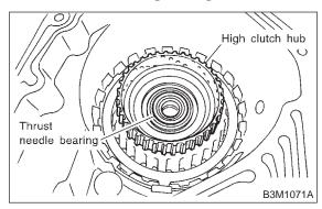
25) Install the high clutch assembly.
