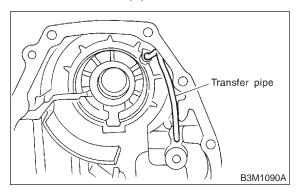
2) Install the transfer clutch assembly to the case.
