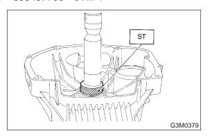
3) Install the differential assembly to the case, paying special attention not to damage the inside of the case (particularly, the differential side retainer contact surface).
