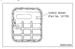
(3) Install the oil pan to the transmission case assembly, and secure with 20 bolts.
