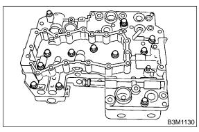
4) Separate the control valve body.
