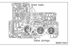
2) Install support plate and upper separate plate to middle valve body.
