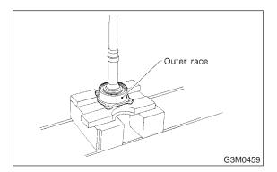
4) Using a press and ST, separate the front roller bearing from the shaft.ST 498517000 REPLACER
