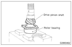
3) After fitting the O-ring to the shaft, attach the drive pinion collar to the shaft.
