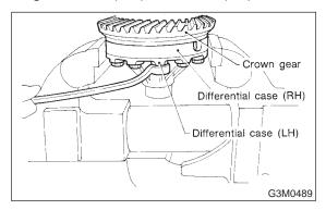
3) Pull out the straight pin and shaft, and remove the differential bevel gear, washer, and differential bevel pinion.
