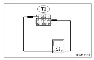
CHECK : Is the resistance less than 1  $\Omega$  in "2" range?
