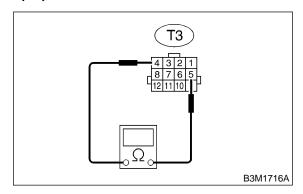
CHECK : Is the resistance less than 1  $\Omega$  in "1" range?
