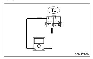
CHECK : Is the resistance less than 1  $\Omega$  in "3" range?
