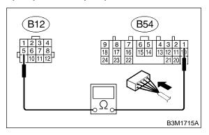
CHECK): Is the resistance less than 1  $\Omega$ ?
