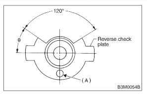
3) Install neutral position switch and back-up light switch to transfer case.
