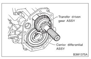
2) Measure height "W" between transfer case and ball bearing on the transfer driven gear.
