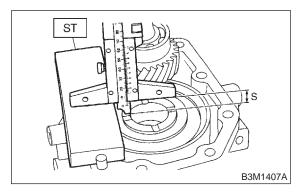
8) Measure depth "T" between extension case and transfer drive gear.
