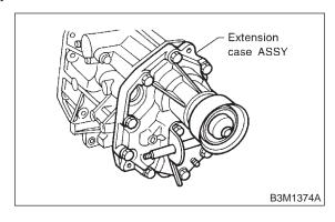
2) Remove transfer driven gear and center differential as a set.
