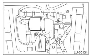
3) Obtain a new oil filter and apply a thin coat of engine oil to the seal rubber.
