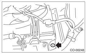
5) Disconnect the radiator outlet hose from the thermostat cover.
