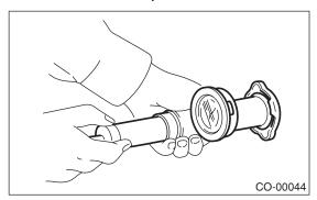
2) Increase pressure until the tester gauge pointer stops. Radiator cap is functioning properly if it holds the service limit pressure for five to six seconds.
