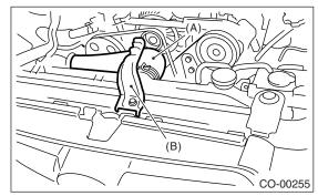
17) Remove the radiator main fan motor assembly from vehicle.
