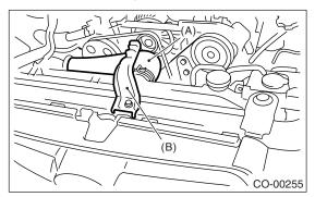
4) Install the mounting bolts of radiator main fan motor assembly.
