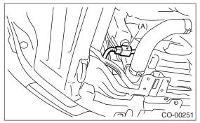
6) Remove the heat shield cover from radiator. (AT model)
