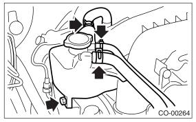
2) Fill with engine coolant. <Ref. to CO(H4DOTC)-13, FILLING OF ENGINE COOLANT, REPLACE-MENT, Engine Coolant.>
